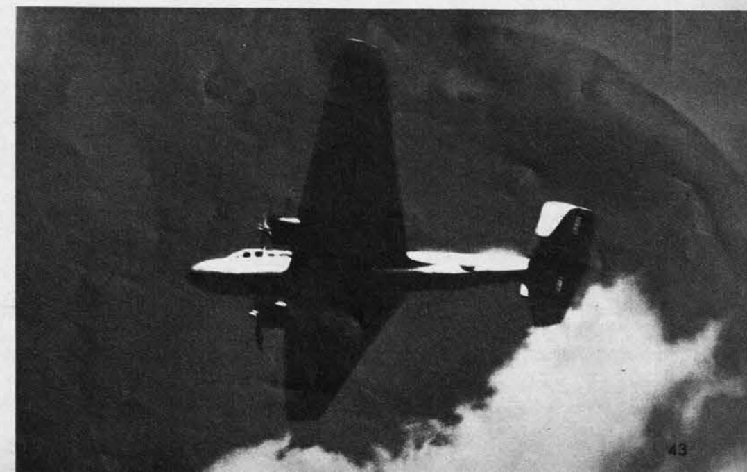
Nell's close-set fins and rudders sometimes appear as one in distant views, are not as quickly visible as B-25's. Fuselage is broken at top by huge blister housing 20-mm. cannon set above trailing edge of wing. Angular wing, tailplane show clearly in picture below.
